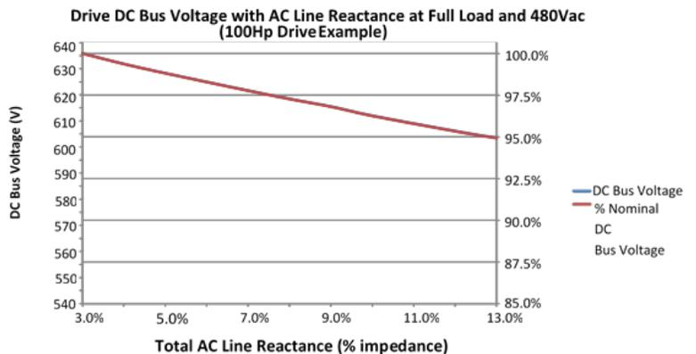
Figure 2: DC Bus voltage at full load output power
