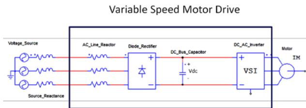
Figure 1: Variable Speed Motor Drive
